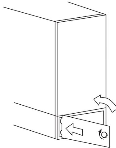
**Fig. 32 - Replace Bottom Filter Cabinet Door**
