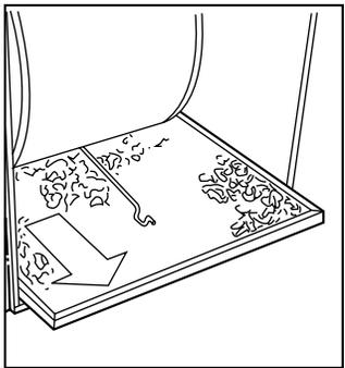
**Fig. 24 - Slide Air Filter Out of Furnace**
