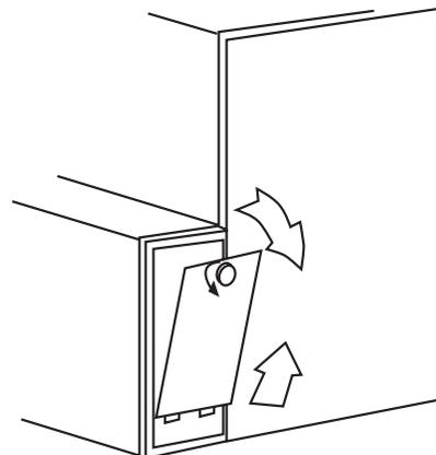
Fig. 21 - Removing Side Filter Cabinet Door
