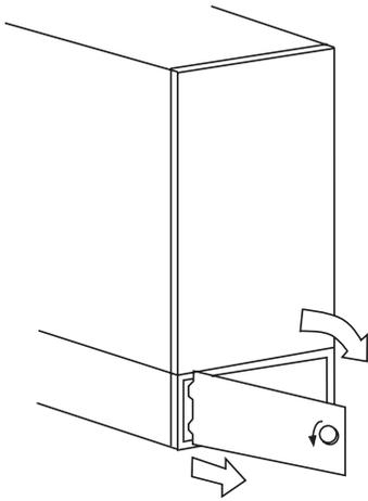
**Fig. 22 - Removing Bottom Filter Cabinet Door**
