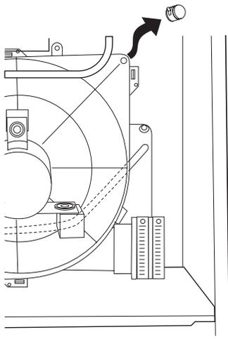
**Fig. 35 - Upper Inducer Housing Drain Connection Cap**
